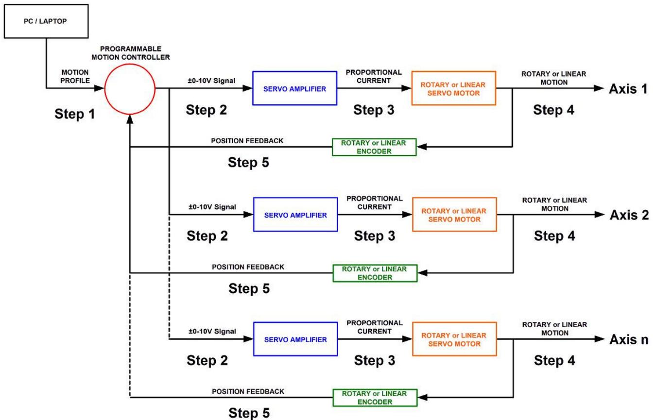
**Step 1.** A program or motion profile will be written on a PC or laptop and downloaded to the motion controller. This program will contain parameters such as speed, acceleration, deceleration, PIDs, desired position, etc...
