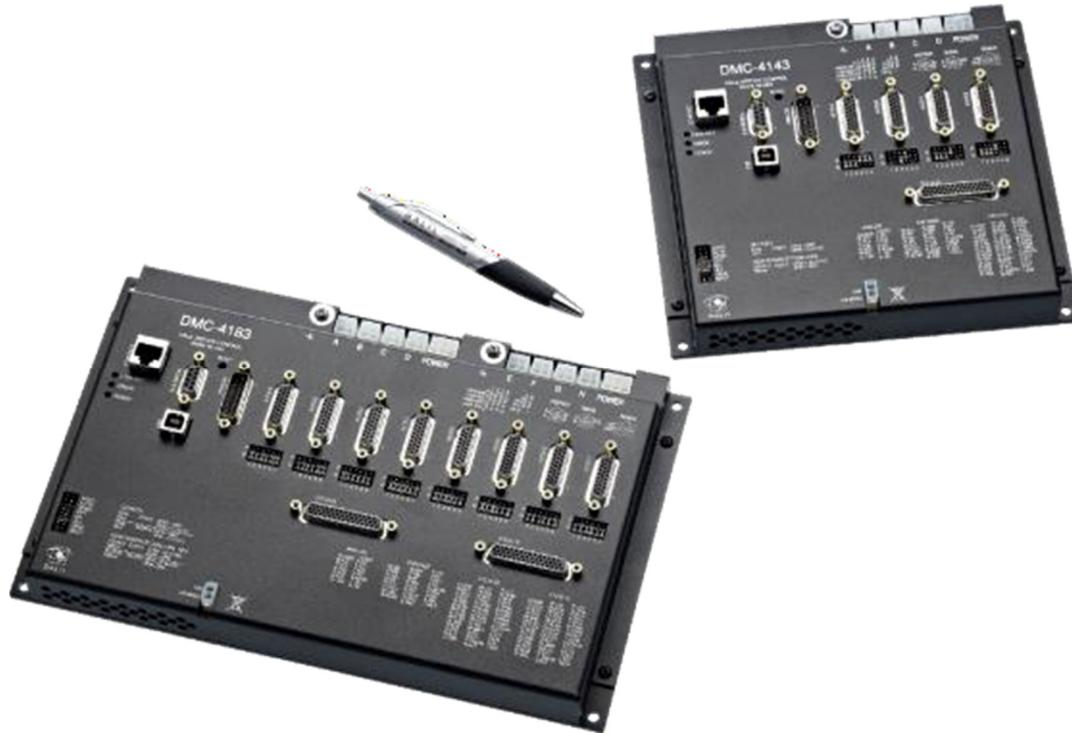
The MCSA-41x3 motion controller is a standalone motion controller.
